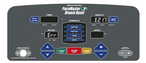
"Err" in the Incline Display - indicates a problem with the elevation system. Note: The treadmill will still function with the "Err" displayed in the incline Display, but the elevation system will not function. To determine the exact error code follow the procedure below.
